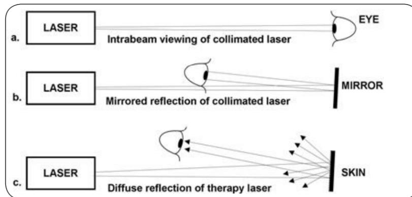
**Figure 3: Conditions of ocular exposure to direct or reflected laser beams.<sup>6</sup>**
