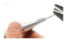
> Bend the optic fiber tip at the notched location. It breaks at the notched location with a smooth, perpendicular fracture surface.
